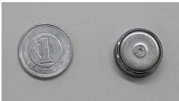
Figure 2. A temperature and humidity sensor used for the inner-bag environment measurement experiments.
