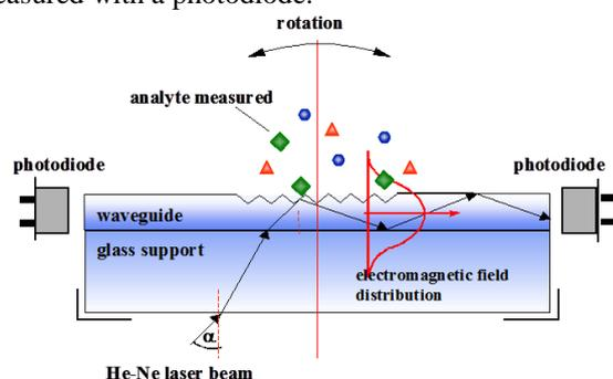
Figure 1. The schematic arrangement of an optical waveguide lightmode spectroscopy immunosensor.
