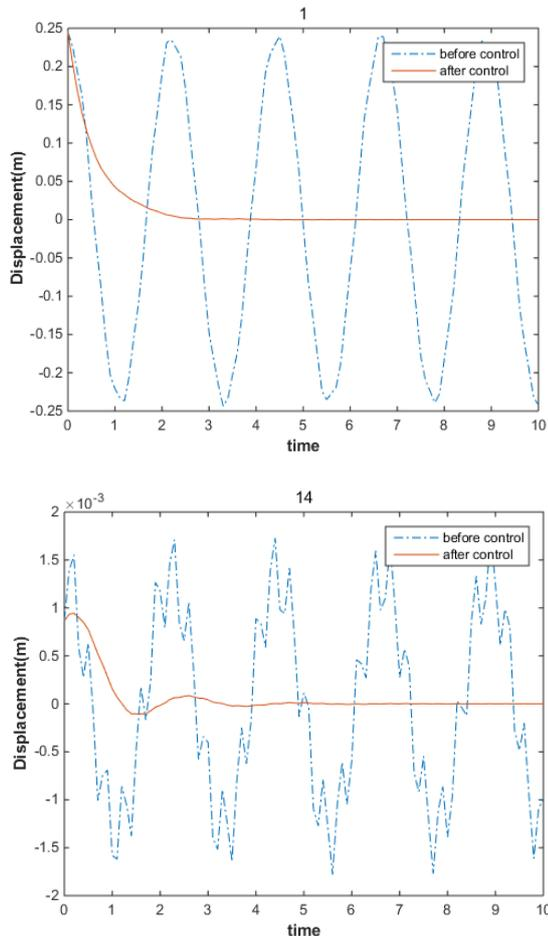
Figure 3. Displacement of Nodes 1 and 14 in the horizontal direction
