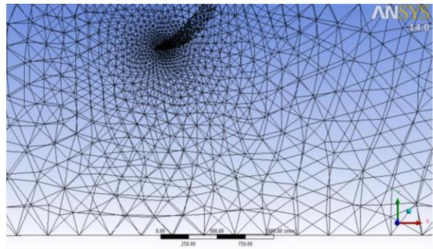
Figure 3. Mesh for flow domain.
