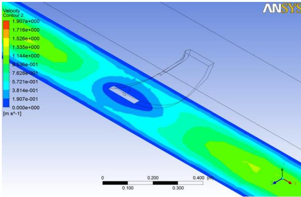
Figure 5. Soil flow through the end leg of a subsoiler.
