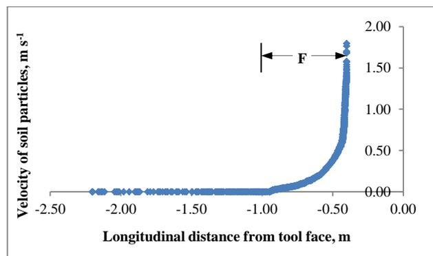
Figure 9. Soil failure front (F) for the moving tool.
