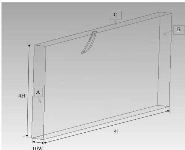
Figure 2. Domain size and boundary conditions by A: Inlet, B: Outlet, C: Free surface
