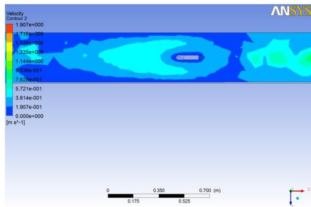
Figure 4. Soil flow around a subsoiler at the free surface (top view of the channel).
