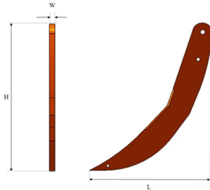
Figure 1. CAD file of subsoiler type curved leg.
