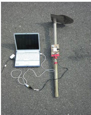
Figure 2. Hoe connected to sensors and laptop PC
