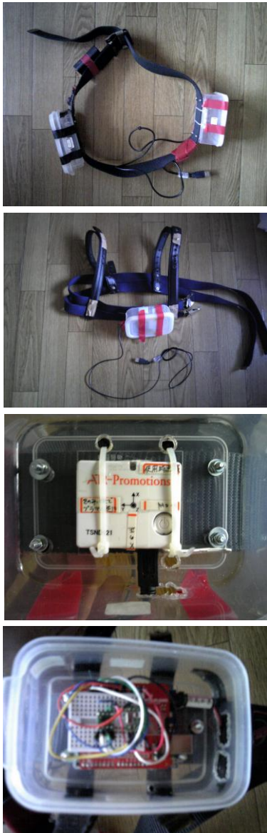
Figure 1. Microcomputers with various devices, store-bought sensing modules, and original vest-shaped and belt-shaped WSs
