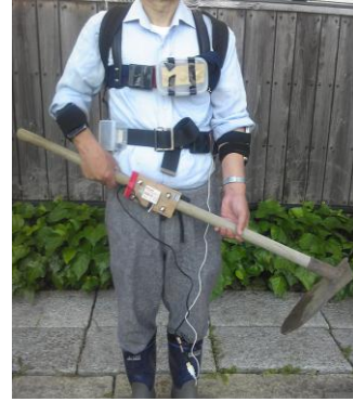
Figure 3. One subject equipped with measuring modules and knapsack with laptop PC connecting to various modules
